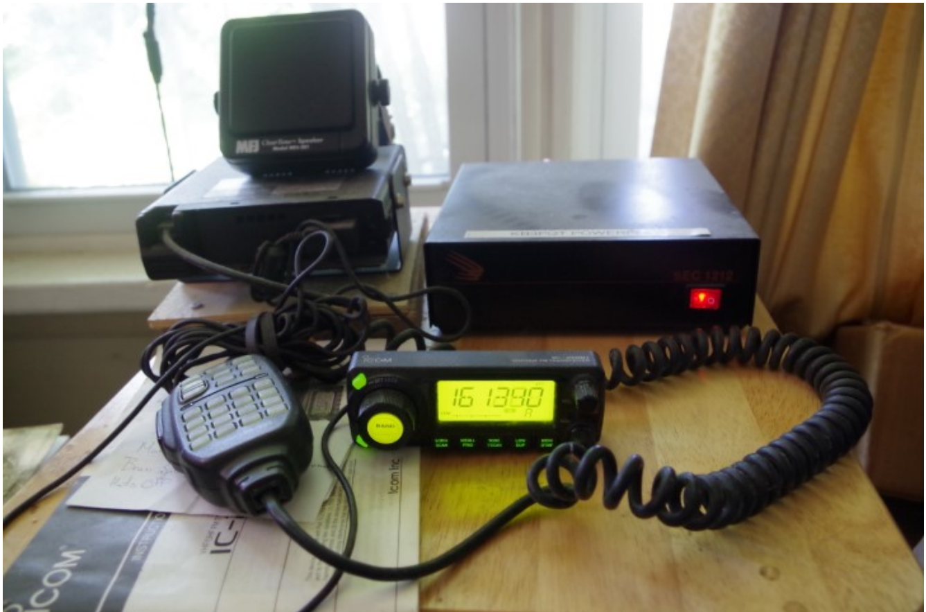
MFJ 1730 2m Jpole (to left of speaker in window) with Icom 208H scanning the 160mhz land commercial railroad frequencies.
