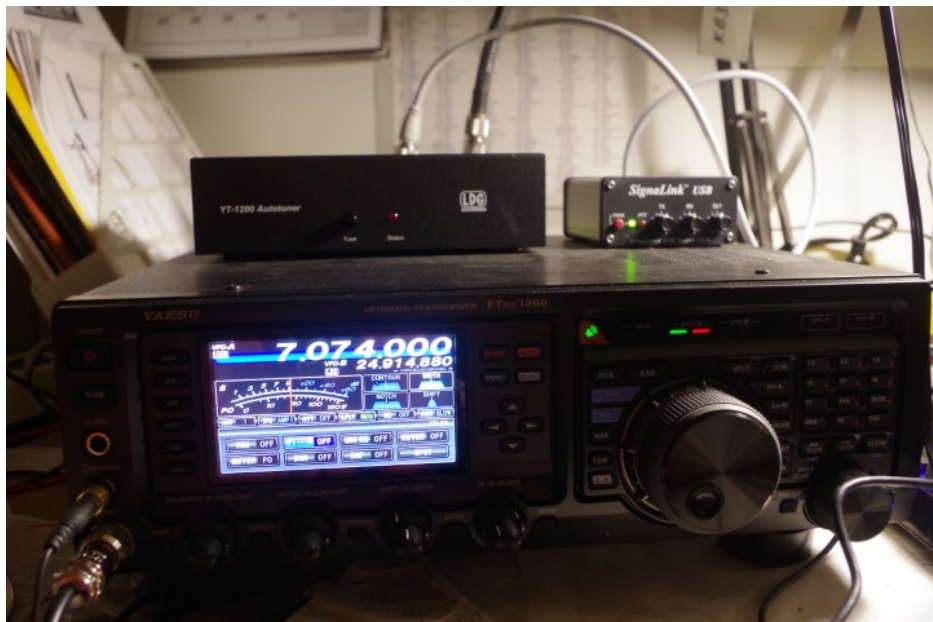
Yaesu FT DX1200 with LDG Y1200 antenna tuner and Signalink USB sound card
