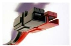
This photo is oriented for the RRTT alignment I described. Other people may have learned an alignment that is rotated 180 degrees from my view. Learn either one. In the long run they end up with the parts properly aligned with the standard.
