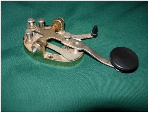
Photo 1 J-38 Straight Key for sending Morse Code
