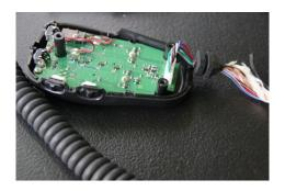
Then I reinstalled the PTT switch, slipped the back cover back on and reinstalled the three screws that had been removed earlier.
