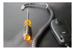
Next I removed the back cover. The Push-To-Talk (PTT) switch fell out, so I laid it to one side. There is a plastic connector where the cord connects to the printed circuit board. I pried it off and slipped the new cord's connector in place and fastened the strain relief.
