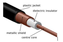
Many of us are familiar with 75 Ohm coax cable used for television and video applications. These typically have a Type F connector. RG-6 and RG-11 and RG 59 are common sizes. We will confine our coax discussion to commonly used radio type cables.
